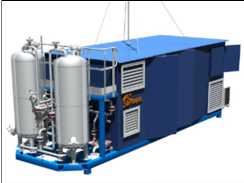
Figure 10 – Skid de purification membranaire du biogaz
